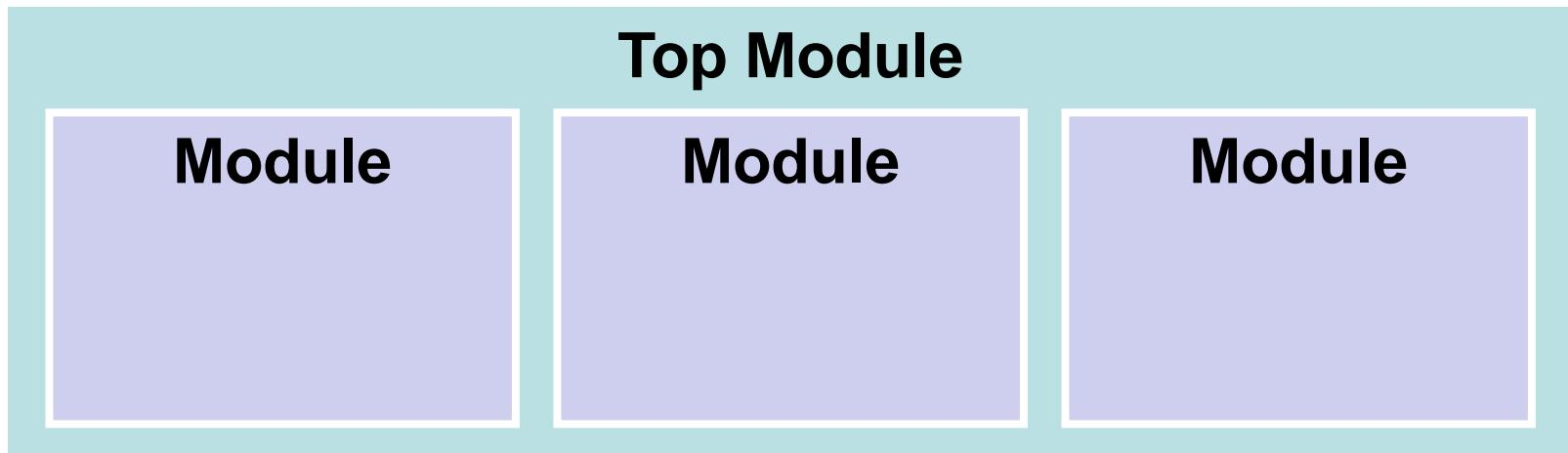
Connected by relating I/O and internal wires
